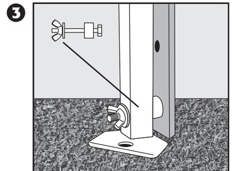
**STEP 3:** Next, tighten **nut & washer** firmly to ensure the bolt is secured with the stake and the leg of the canopy.
