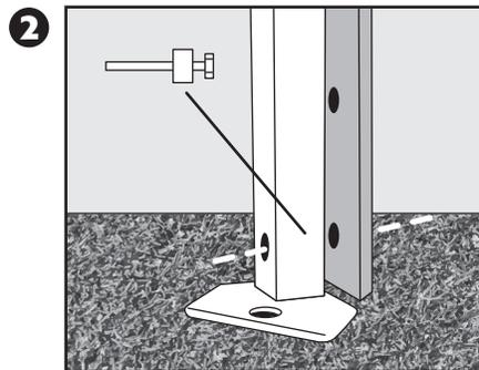
**STEP 2:** Line up stake (hole) with canopy leg (hole). Once the holes are aligned, insert the **bolt & spacer** through the stake into the Z-Shade canopy leg.
